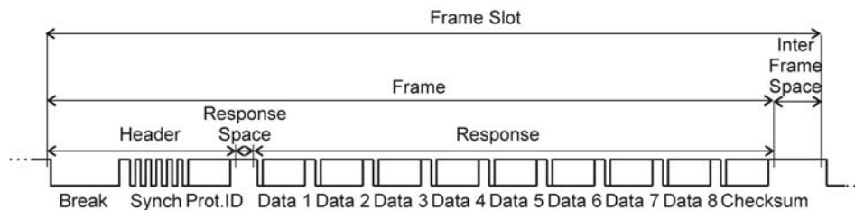
Figure 2.5: Structure of a LIN Frame[LIN03]
